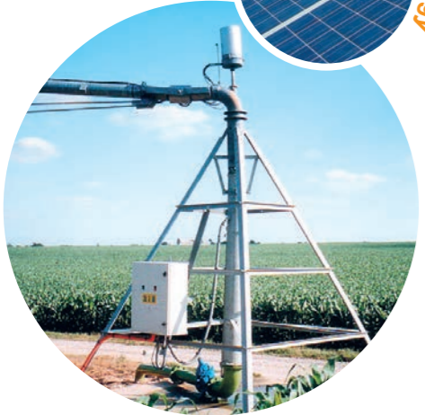
Fixed or towable the center is anchored to a concrete base.
